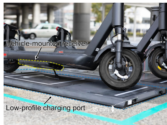
Fig. 1 A capacitive coupling-based wireless charging system, showing the 35 mm low-profile charging port on the ground and the vehicle-mounted receiver under the scooter.
