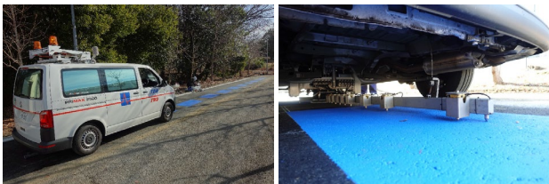
Fig.4 The FWD test scene
