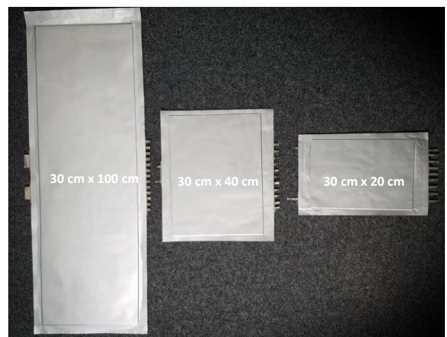
Fig. 4 Manufactured bipolar cell sample formats.
