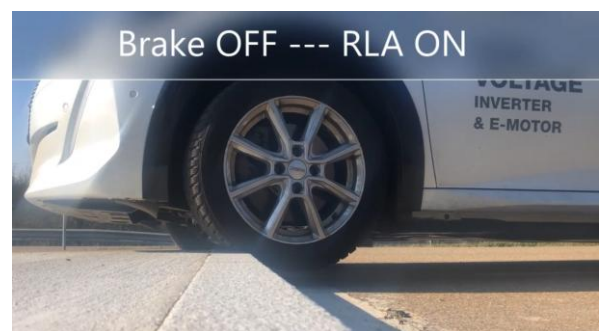
Fig. 14 Test vehicle with integrated Rotor Lock Actuator (RLA) on front axle e-drive parked on the edge of a curb stone (no ground level wheel contact)
