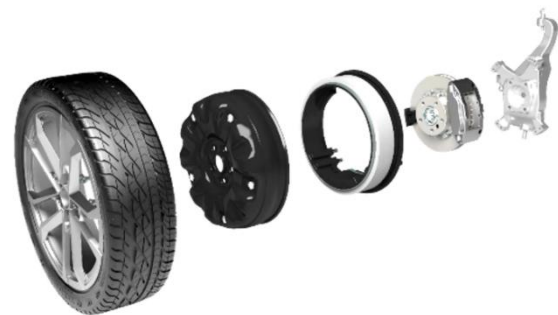
Fig. 1 Standard Elaphe direct drive motor layout with integrated friction brake
