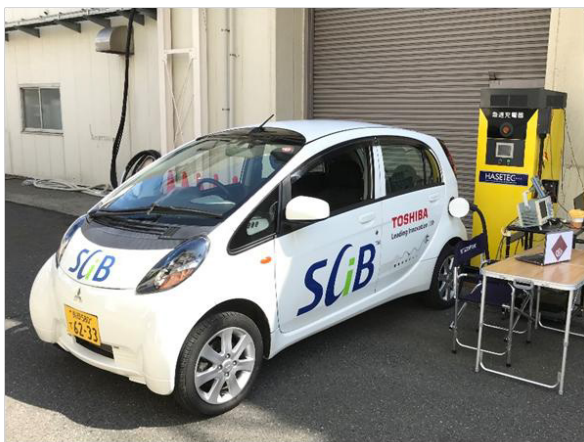
Fig.2 Photo of field-test that EV was diagnosed by SC-EIS method installed into the CHAdeMO charger
