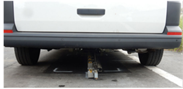
Fig.4 FWD measurement on pavement with embedded coils
