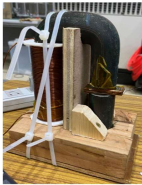
Fig. 6 Photograph of an experimental set-up of eddy current loss of NdFeB laminated permanent magnet.
