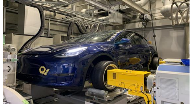
Fig. 3 Test vehicle in chassis dynamometer setup
