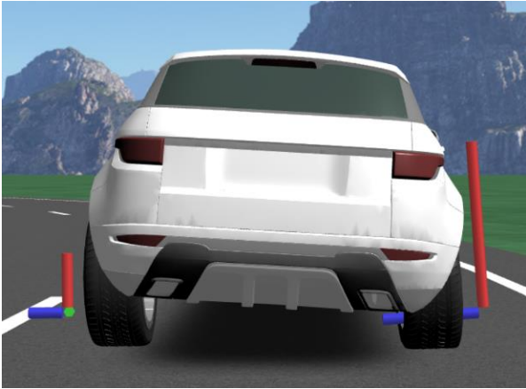
Figure 5. The vehicle rolls during the cornering maneuver, with the wheel cambered into a turn.
