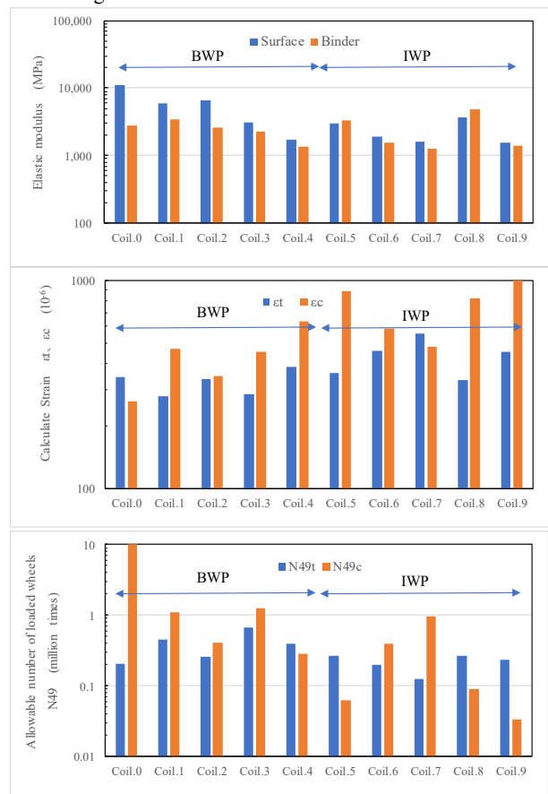
Fig.6 Comparison of the layer elastic modulus of each layer, calculated strain, and allowable number of load cycles
