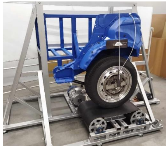
Figure 7: HIL environment with installed wheel corner.
