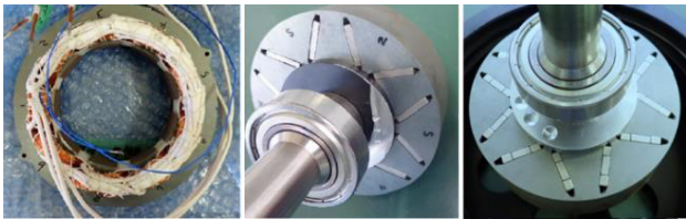
Fig. 3 Stator (left), single magnet rotor (middle), and joined magnet rotor (right).
