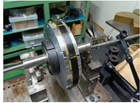
Fig. 11. Photograph of the prototype rotor.
