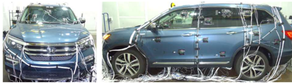
Figure 1: Test Vehicle with Sensors Applied
